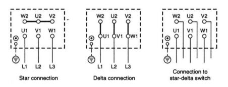
For special voltages and the like, different connections will be noted on the motor nameplate beside the voltage.
